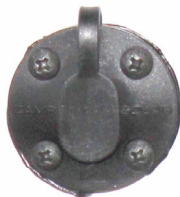
Single Solar Port (Located on driver side of motorhome)
