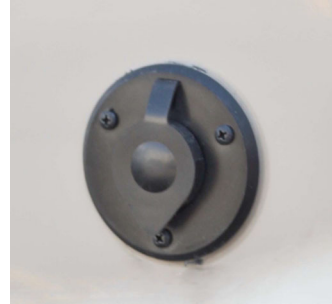
Cable TV Connection (Located on driver sidewall) -Typical View
