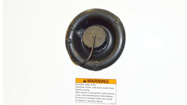
Water Tank Gravity Fill -Typical View
