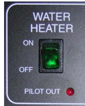
Gas Water Heater Switch (Located on Systems Monitor Panel)
