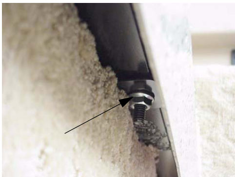
Hydraulic Pump Access (Remove nut from bolt on underside of step and lift off step) - Typical View
