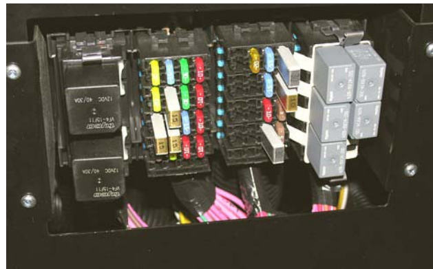
Automotive Fuses (cover removed) - Diesel
