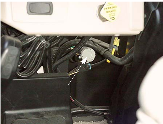
Diagnostic plug on steering column support beneath left side of dash (Freightliner® and Workhorse™ Chassis) -Typical View
