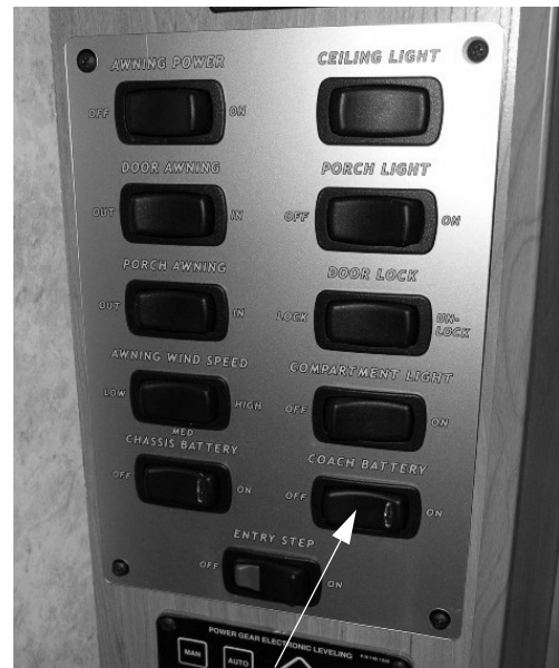
Auxiliary Battery Switch (Located near entrance door) -Model M39N shown
