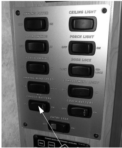
Chassis Battery Disconnect Switch (located inside the entrance door) -Model M39N shown
