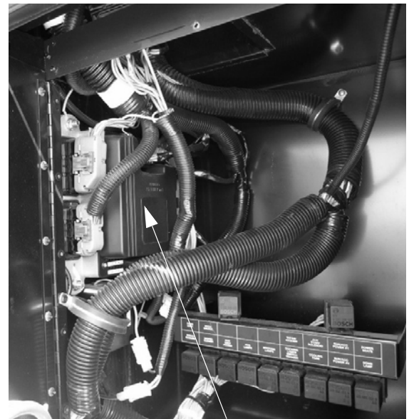
Front Chassis Control Module - CCM (Shown with panel removed)
