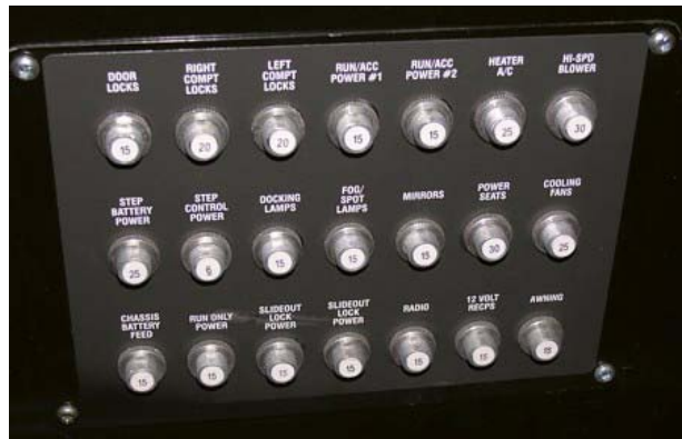
Automotive Circuit Breakers – push to reset (Breakers are labeled for components equipped)
