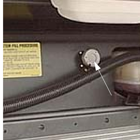
Diagnostic plug on rear engine compartment shroud (Freightliner® Chassis only) -Typical View
