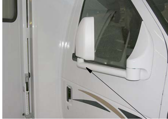
The mirrors can be folded back against the cab doors if needed.
