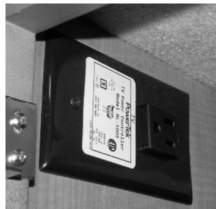
Front TV Ignition Switch Interlock -Typical View
