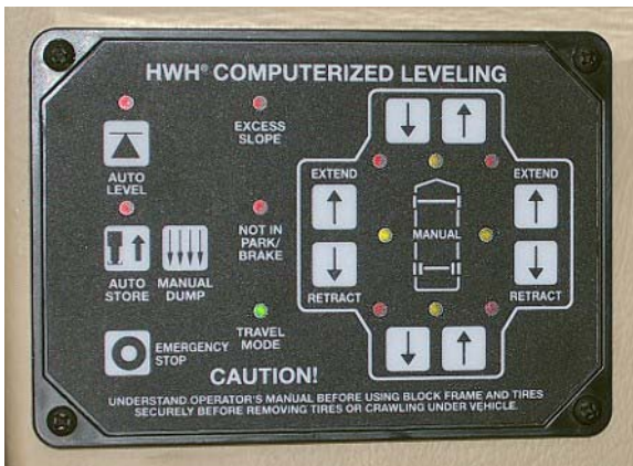
Leveling System Control Panel
