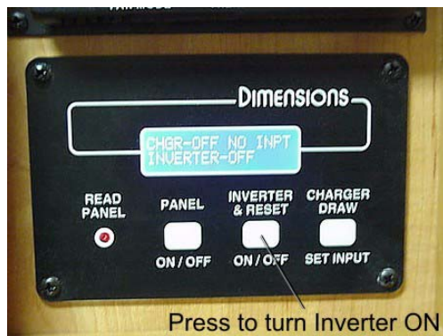
Inverter/Charger Control Panel
