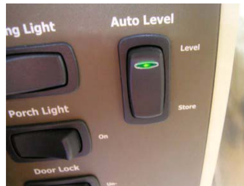
Auto Level Switch inside Entrance Door
