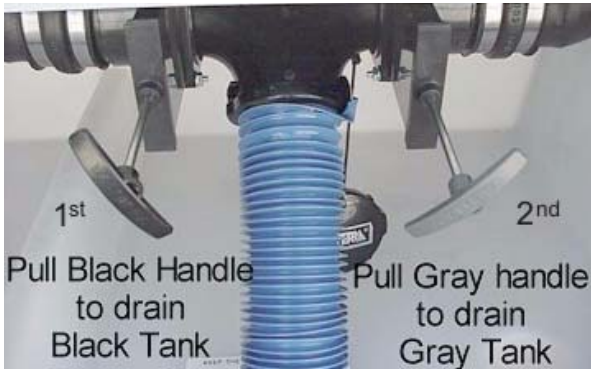
Holding Tank Valves (Typical)
