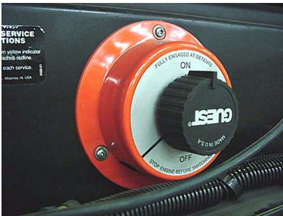
Chassis Battery Cutoff Switch inside rear engine access grille
