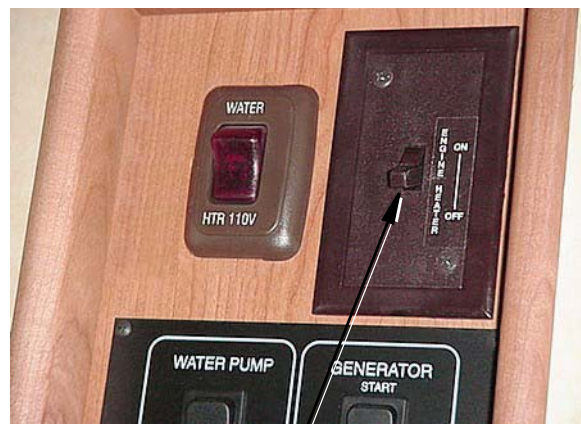
Diesel Engine Heater Switch (typical)
