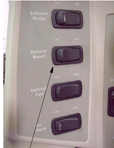
Battery Boost Switch
