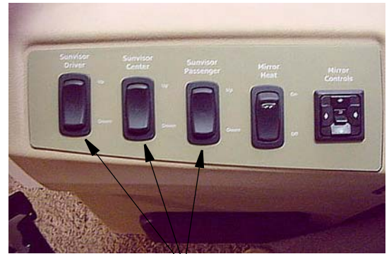
Driver Side Sunvisor Switches (center visor not equipped on models 40FD & 40TD)
