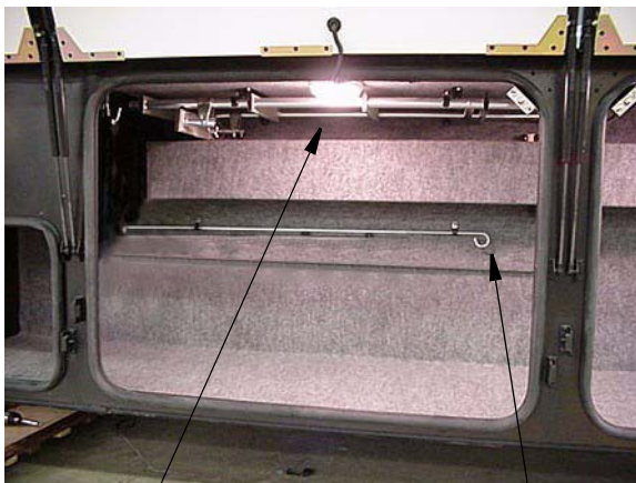
Roof Ladder Extension
