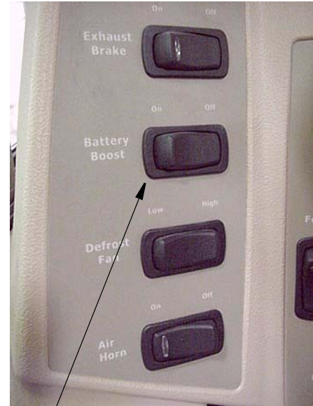
Battery Boost Switch
