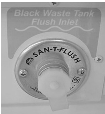
Black Water Tank Flush Inlet (Located in water service center) -Typical View
