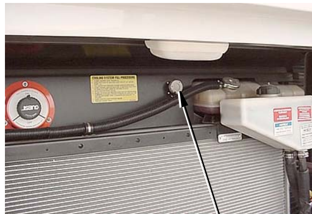
Diagnostic plug on rear engine compartment shroud
