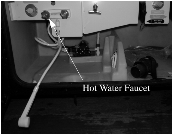
Hot Water Line Drain Valve in Water Service Center (Exterior Shower)
