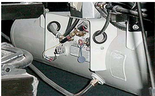
Propane Gas Tank behind slideout room
