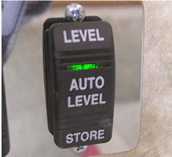
Auto Level Switch inside Entrance Door
