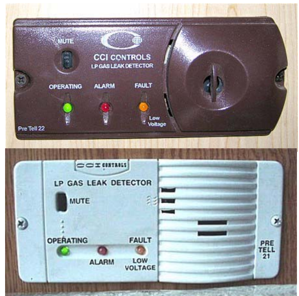
Propane Gas Leak Detectors (typical)
