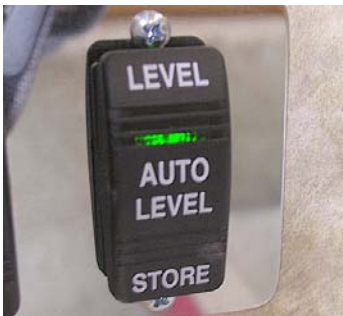
Auto Level Switch inside Entrance Door
