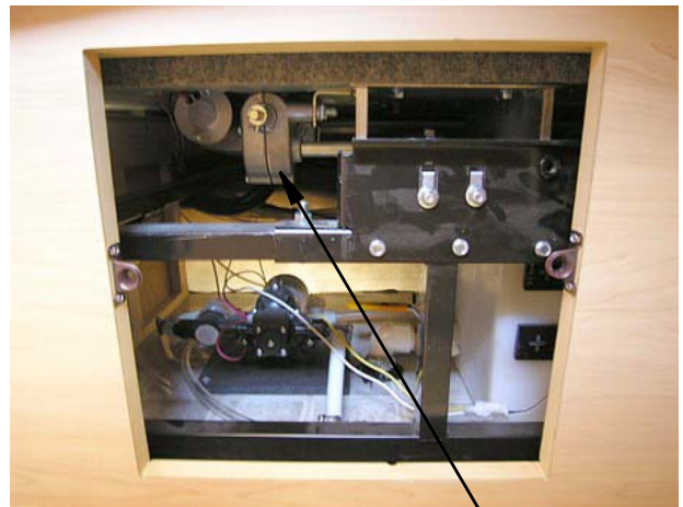
Rear Slideout Motor/Gear Location behind pull-off panel at foot of bed base Model 29H only
