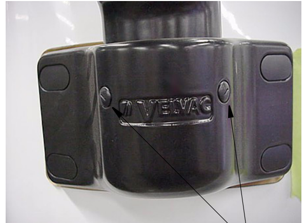
Remove (unscrew) caps to access set screws*
