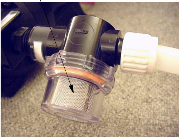
Water Pump Strainer
