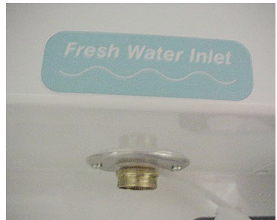
Fresh (City) Water Inlet
