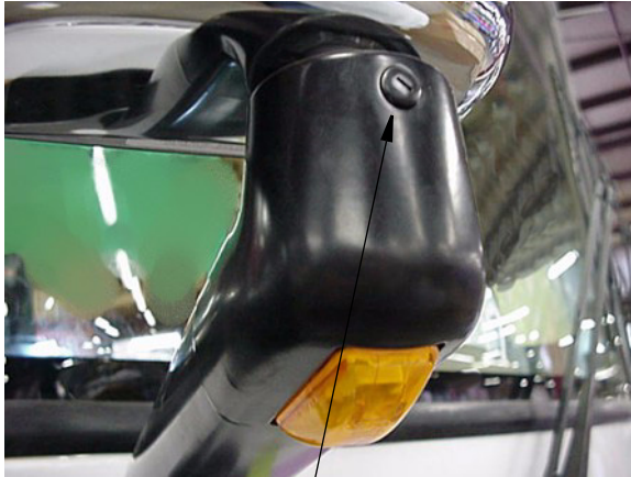
Mirror Arm Unscrew protective cap and loosen Allen head set screw to pivot mirror head.
