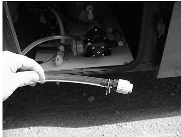
RV Antifreeze Draw Tube in water center or near water pump (insert into container of RV water system antifreeze)
