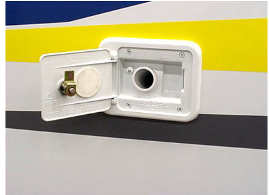
Water Tank Gravity Fill (typical)
