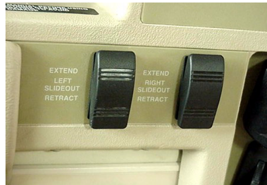
Front Slideout Switches on dash
