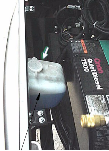
Windshield Washer Reservoir behind front "hood" panel.
