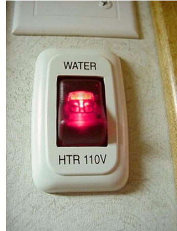
Electric Water Heater Switch (Typical)
