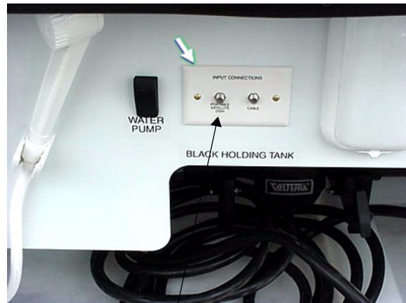
Exterior Connection for Satellite Dishes and Cable TV (In Water Center Compartment)
