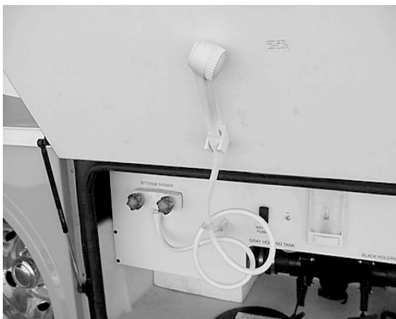
Exterior Shower/Wash Station (Typical)
