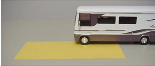
Weighing Left Front 'Corner'
