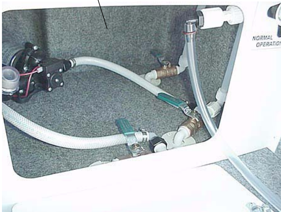
Water Line Drain Valves - Model 39F Behind access panel in small compartment forward of water center
