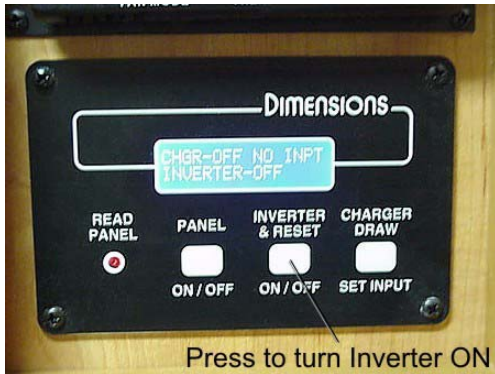
Inverter Charger Control Panel
