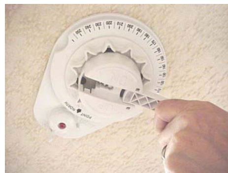
Digital Satellite Dish Control located on ceiling
