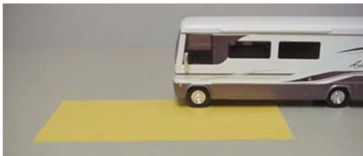
Weighing Left Front 'Corner'
