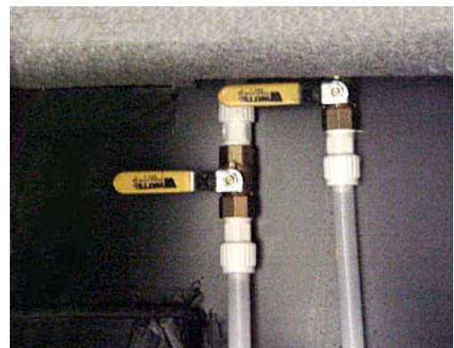
Models 34H & 36G: Water Line Drain Valves in Water Center
