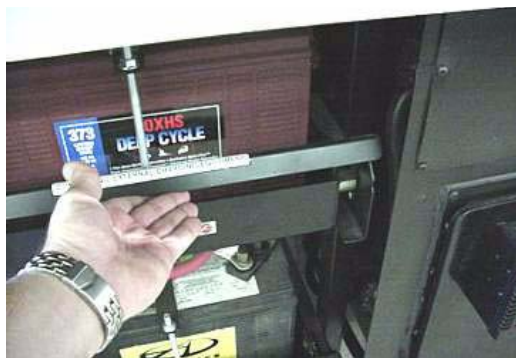
Lift Battery Tray Retainer Latches
