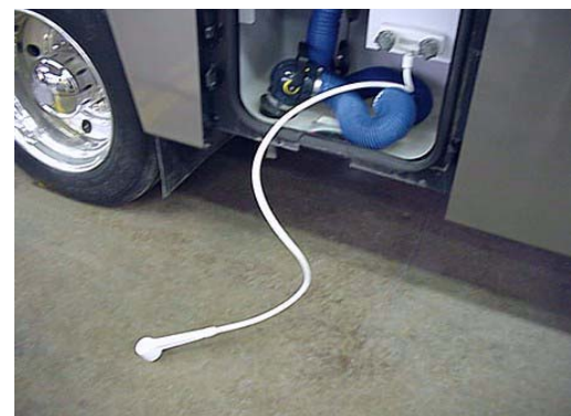
Models 34H & 36G: Water Line Drain Valves in Water Center
