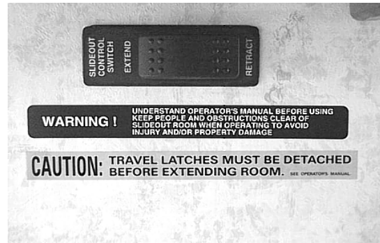
Rear Slideout Switch (on wall in rear of couch - varies by model)
