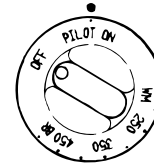
Oven Control Knob in "PILOT ON" position
