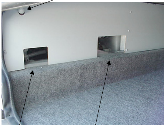
Winterizing Valve and Water Tank Drain Valve Access in RH Storage Compartment
