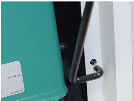
Generator Door Prop Rod (insert into hole in door frame)
