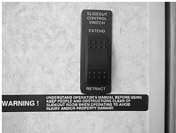
Rear Slideout Switch (on wall in rear of coach)
