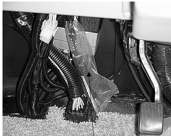
CB Wires (in plastic sheath)
