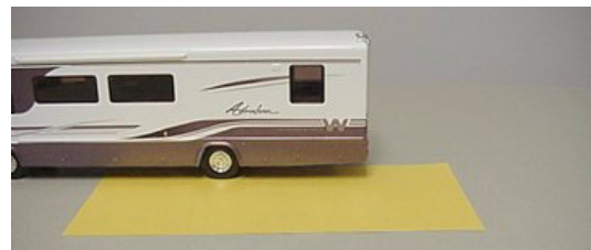
Weighing Left Rear ‘Corner’
