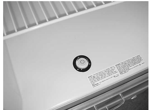
Place bubble level in bottom of refrigerator
