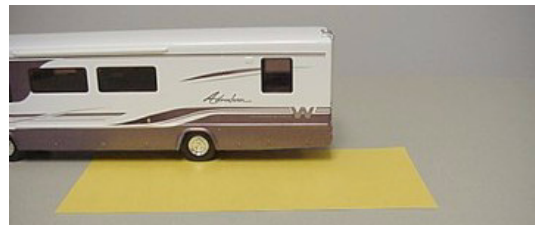
Weighing Left Rear ‘Corner’
