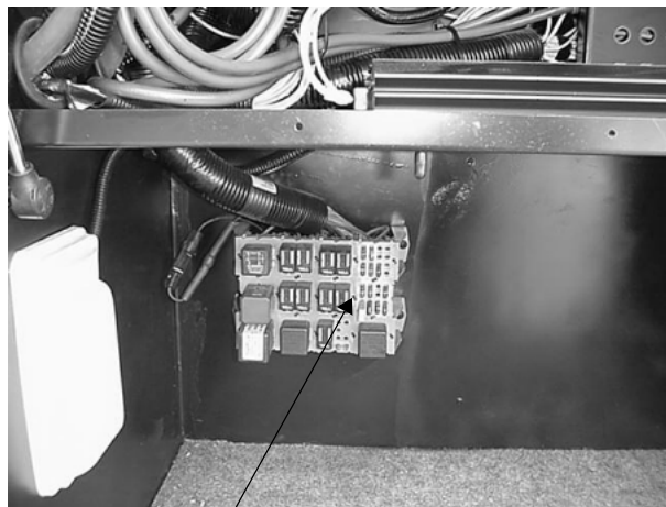
Automotive 12-Volt Fuse Panel
