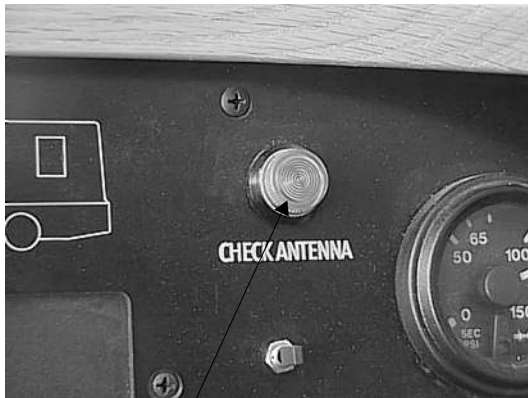
“Check Antenna” Light
