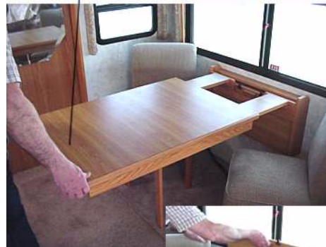
Lift end of table slightly and pull out from wall
