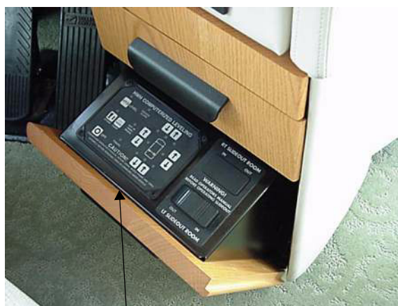
Automatic Leveling System Control Panel
