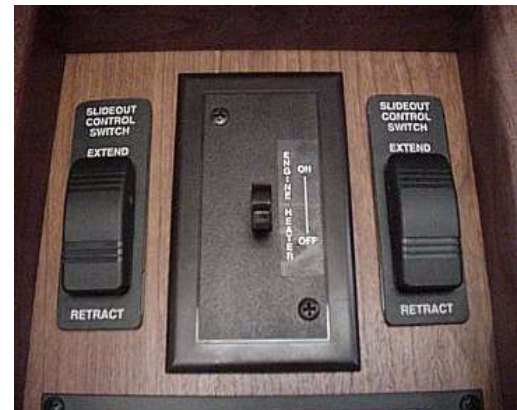
Diesel Engine Heater Switch
