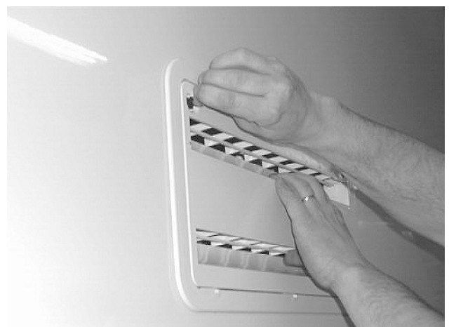
Turn latches open with coin
