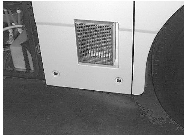
Water Heater Service Access Panel
