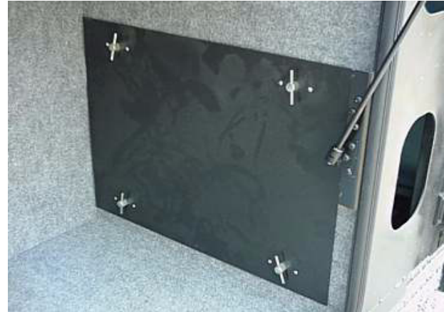
Slideout Pump Access Panel inside StoreMore compartment
