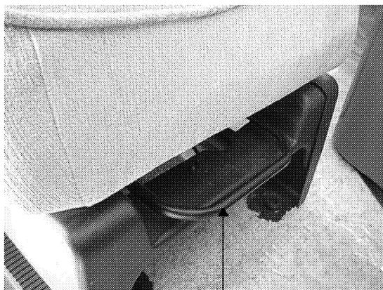
Seat Position Adjustment Bar (Lift to slide foward - back)
