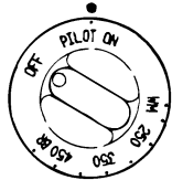
Oven Control Knob in "PILOT ON" position
