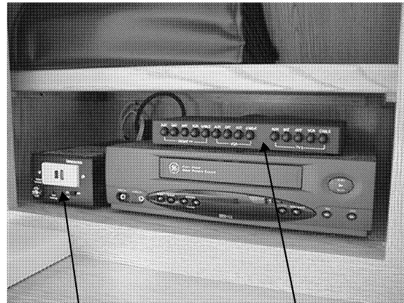
DC/AC Inverter Video Selector System
