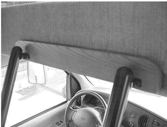
Front Bunk Ladder Shown hooked into mattress bracket
