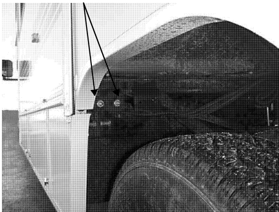
Rear Helper Spring Air Valves located inside left rear wheelwell
