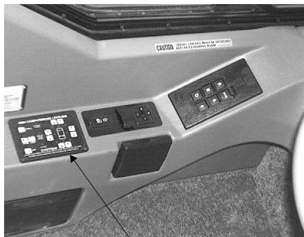
Automatic Leveling System Control Panel
