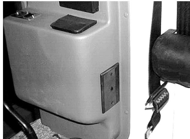
Front Phone Jack: On rear facing end of the passenger sidewall armrest just behind the copilot seat.
