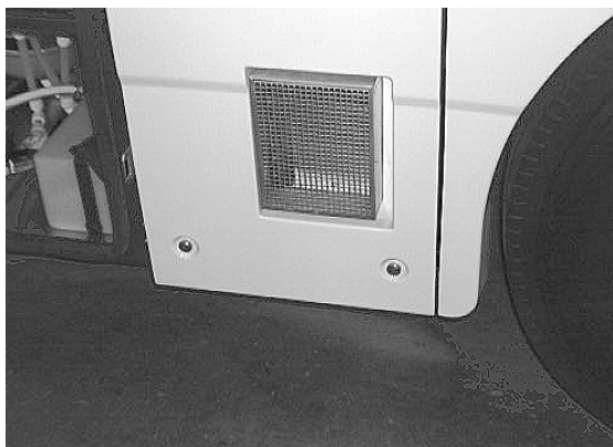
Water Heater Service Access Panel
