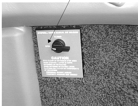
Emergency Position - Open (Normal - Closed)
