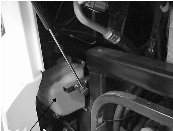
Windshield washer reservoir inside front “hood” compartment
