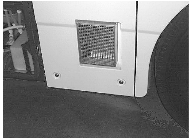
Water Heater Service Access Panel
