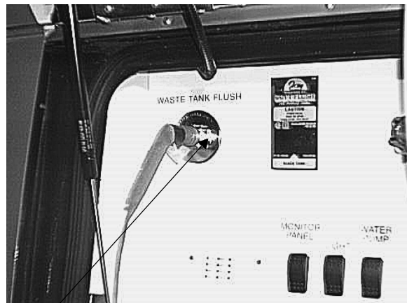
Flushing System Inlet
