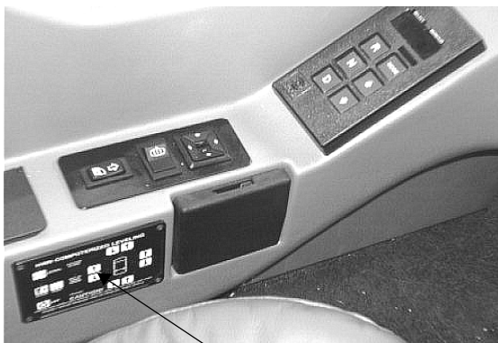
Automatic Leveling System Control Panel
