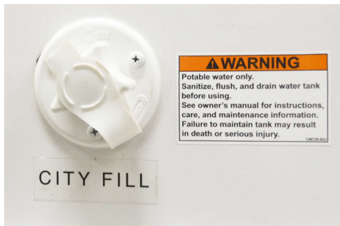
Fresh (City) Water Inlet -Typical View
