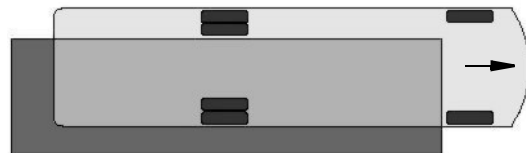
Weighing Right Rear Corner
