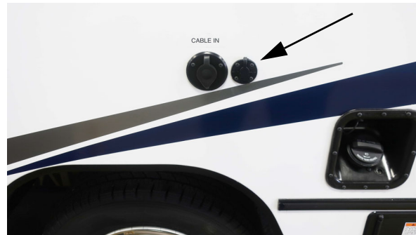
Single Solar Port (Located on driver side exterior sidewall) -Typical View
