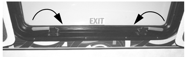
Escape Window (Lift both red safety latch handles UP and push window OUT) -Typical View
