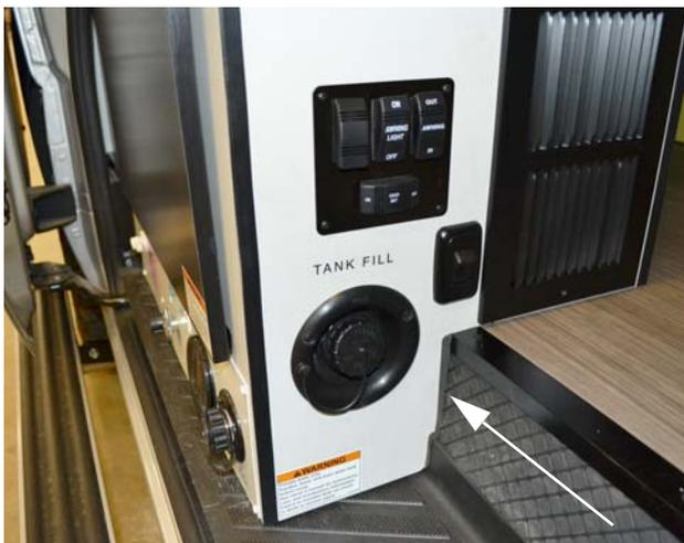
Water Tank Gravity Fill
