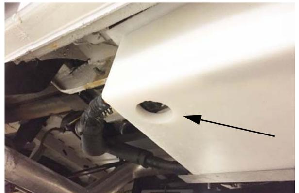
**Water Tank Drain Plug**
