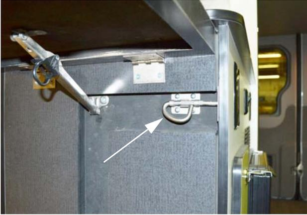
5. Firmly grasp both sides of countertop extension and pull away from galley and lower to the floor and close the sliding door.
