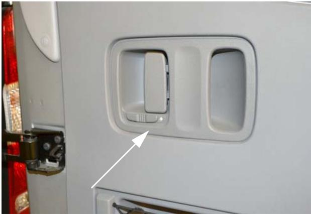
2. On passenger side door, pull latch forward and push door open.
