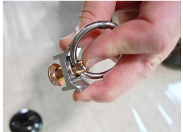
2. Slide tie-down ring into the floor bracket, then release the top of the tie down ring to secure into the floor bracket.
