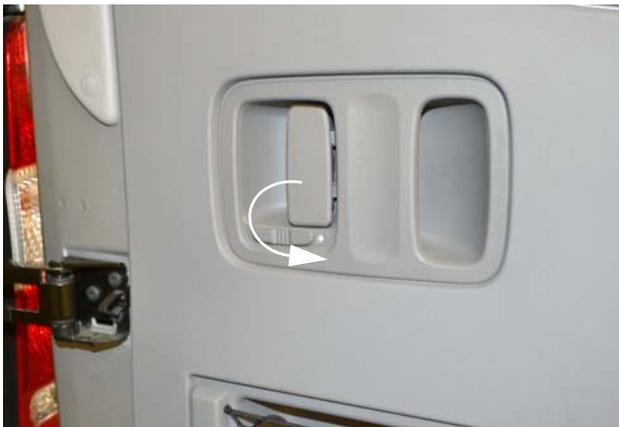
*NOTE: The rear passenger side door must be open before opening the rear driver side door.*
