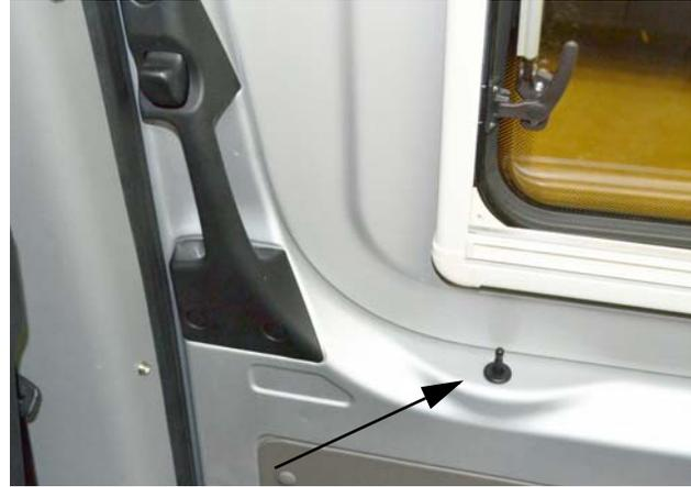
2. To open the passenger side sliding door, push down on the release button on the left-hand side of the door while pushing door outward and sliding to the right.
