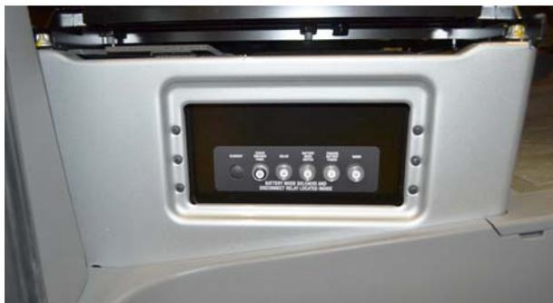
Automotive Chassis 12-Volt Circuit Breakers
