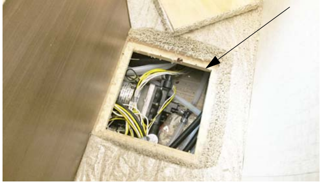
Water Pump (Located beneath removable access panel in bedroom floor on driver side front of bed) -Model 24G shown
