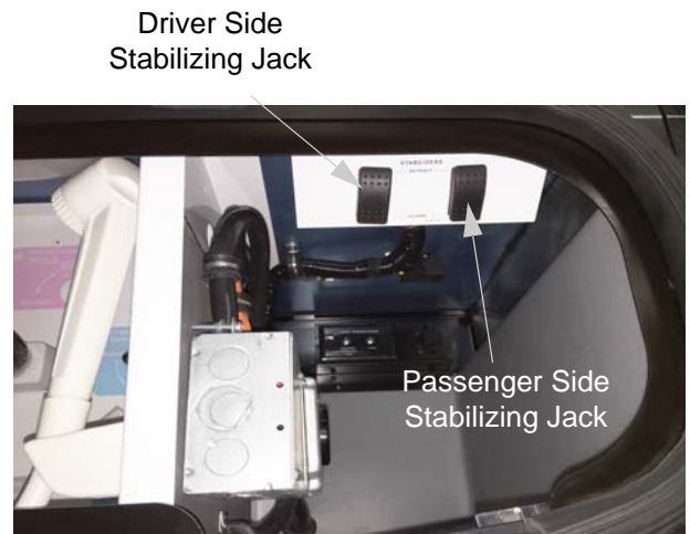
Stabilizing Jack Switches (Located in driver side rear compartment) -Typical View
