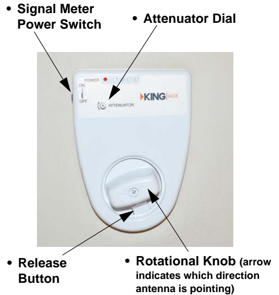
Digital Antenna Signal Meter (Located on ceiling)
