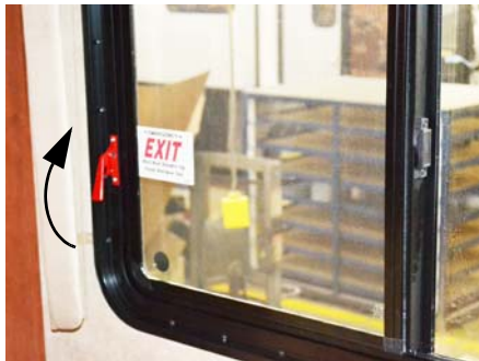
Escape Window (Lift both red safety latch handles UP and push window OUT) -Typical View
