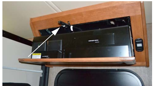
HDMI Cable (Located in cabinet above entrance door) -Typical View
