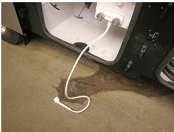
Using exterior shower to drain waterline -Typical View
