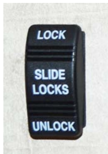
Slideout Room Travel Lock (Your coach may be equipped with one or more types) -Typical View
