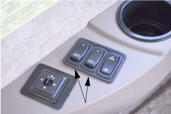
12-Volt Front Drop-Down Solar/ Night Shade Switches (Located on driver side trim panel) -Typical View
