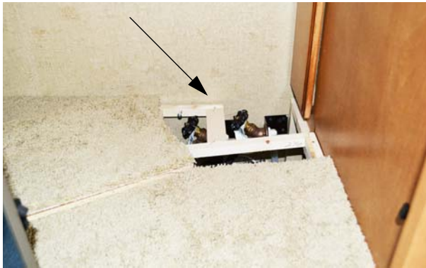
Water Supply Faucets (Located beneath access door in the wardrobe floor.) * Model 35G shown
