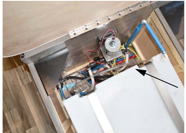
Water Pump (Located beneath bed - extend rear bed slideout, remove mattress from bed, and lift hinged bed board to access) *Model 26A
