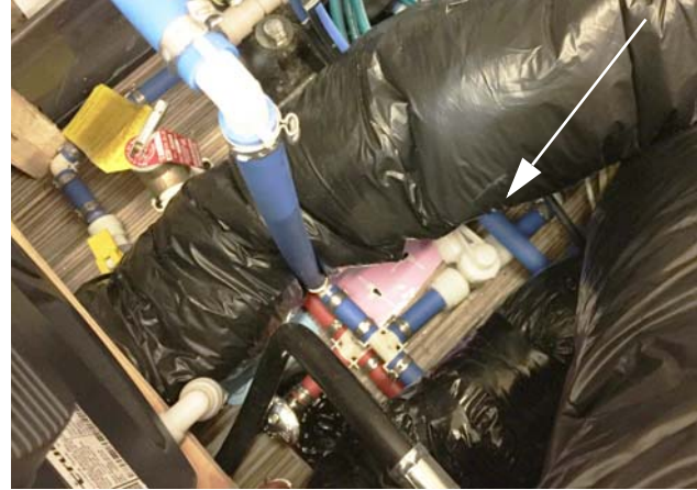
Water Heater Bypass Valve (Located beneath driver side dinette seat)
