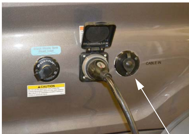
Cable TV Input Connection (Located on the driver sidewall)
