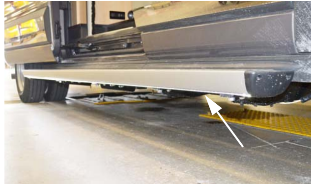
Accent LED Light Strips (Located on passenger side running board) -Typical View
