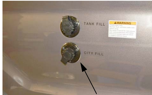
City Fill Inlet (Located on the left sidewall) -Typical View
