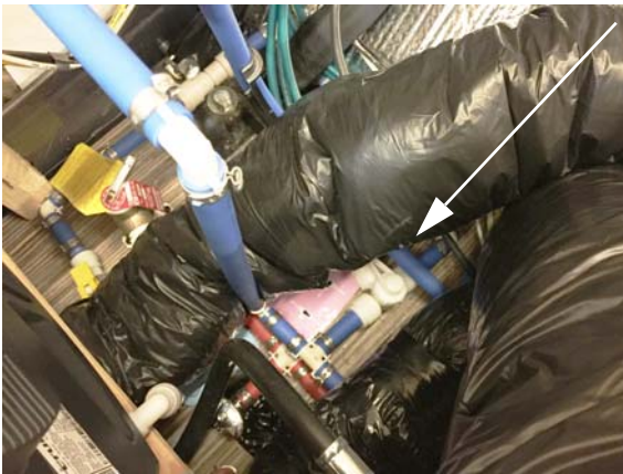
Water Heater Bypass Valve (Located beneath driver side dinette seat)
