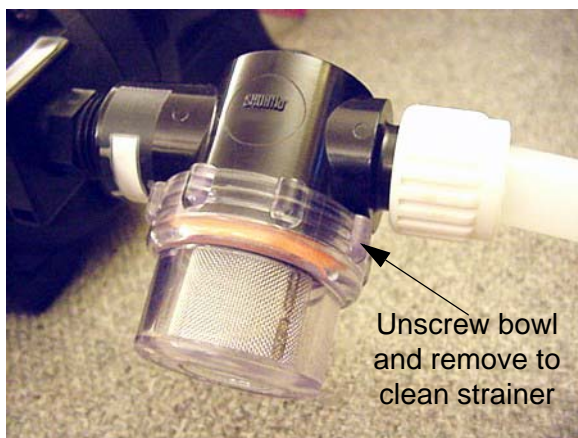
Water Pump Strainer -Typical View
