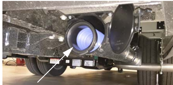
Sewage Drain Hose (Located beneath passenger rear coach)
