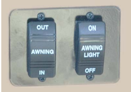
Power Awning Switch and Awning Light Switch (if equipped) (Located at front of galley) -Typical View
