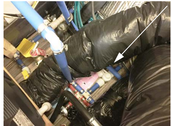
Water Heater Bypass Valve (Located beneath driver side dinette seat)
