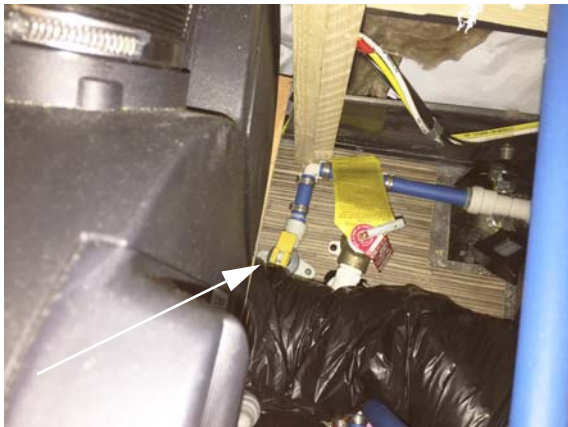
Water Heater Drain Valve (Located beneath driver side dinette seat)
