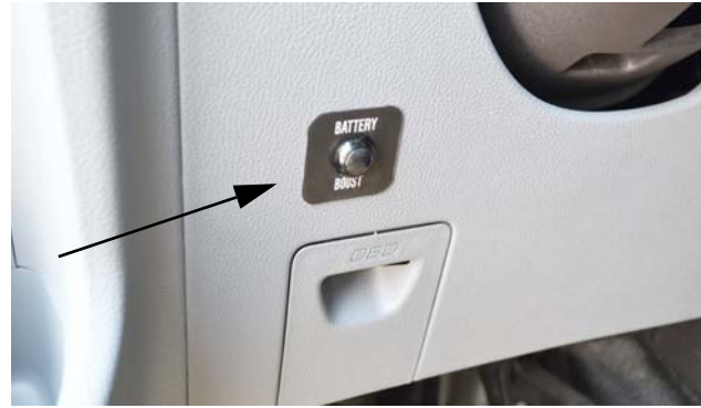
Battery Boost Switch (Typical View - depending on model)
