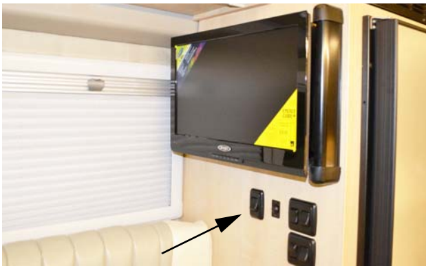
12-Volt TV Master Power Switch (Located on rear refrigerator wall below TV)
