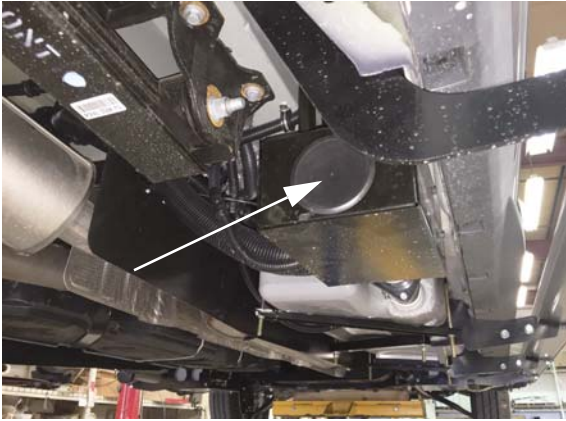
Waste Pump Enclosure (Located on passenger side beneath coach)
