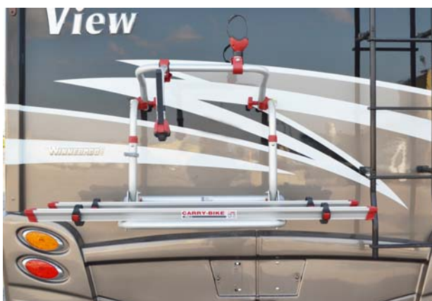
Pull straight down to lower bike rack for use. (shown in down position)
