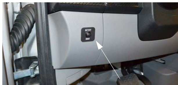
Battery Boost Switch (Located on lower driver side dash)
