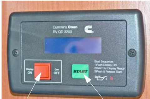
Press to Stop/Prime Press to Start Diesel Generator Start/Stop Buttons (Located near monitor panel) -Typical View
