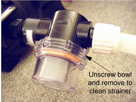
Water Pump Strainer -Typical View
