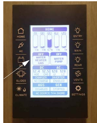
Water Heater Switch
