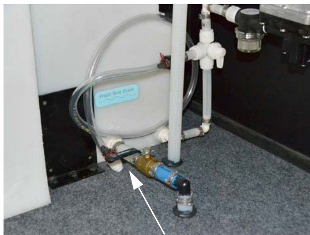
Water Tank Drain Valve (Located in passenger side compartment) *Model 38W shown
