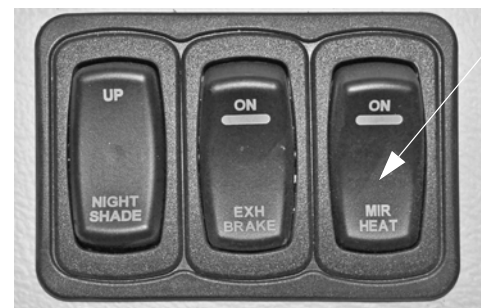
Mirror Heat Switch (Located on dash) -Typical View
