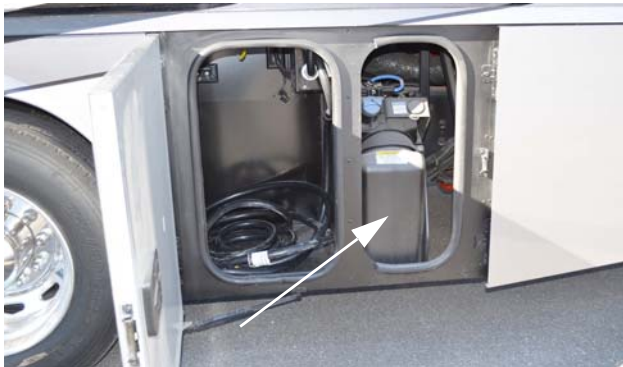
Diesel Exhaust Fluid Fill Tank (Located in driver side compartment behind rear wheel) -Typical View
