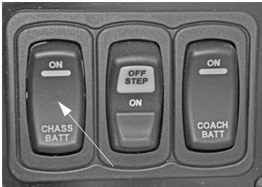
Chassis Battery Disconnect Switch (Located near entrance door) -Typical View
