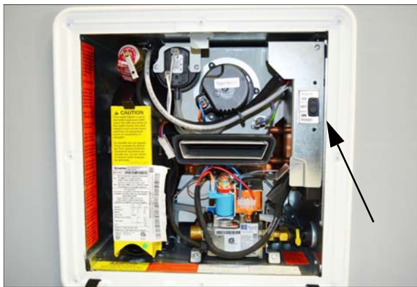
Water Heater Power Switch (Located behind water heater access panel on exterior of coach)
