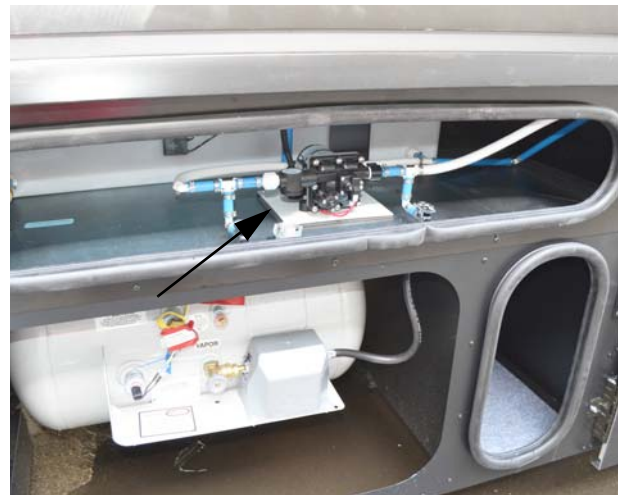
Water Pump (Located in driver side front compartment) *34T Shown
