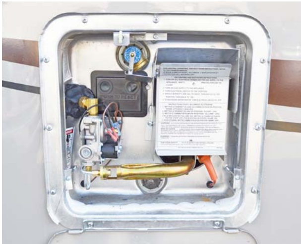
Water Heater Exterior Service Access
