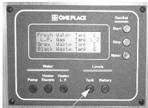
Tank Levels Switch
