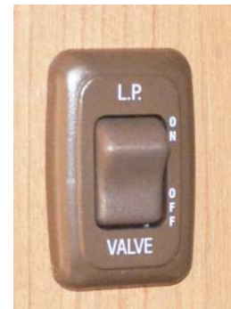
LP Tank Valve Switch
