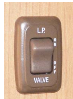
LP Tank Valve Switch
