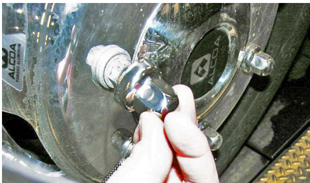
Remove the push on nut covers.
