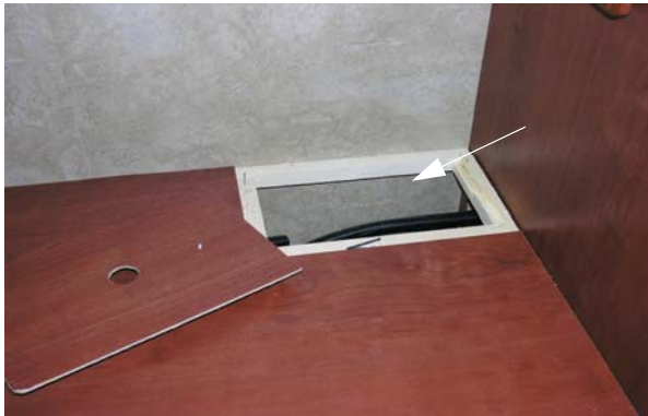
Water Supply Faucets (Located below access panel in wardrobe) * Model 38Q shown
