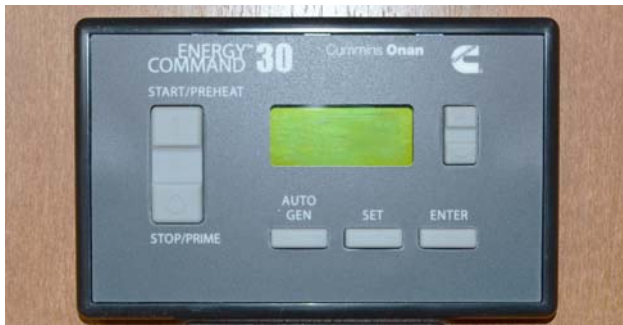
AGS Control Pad (Located near monitor panel)
