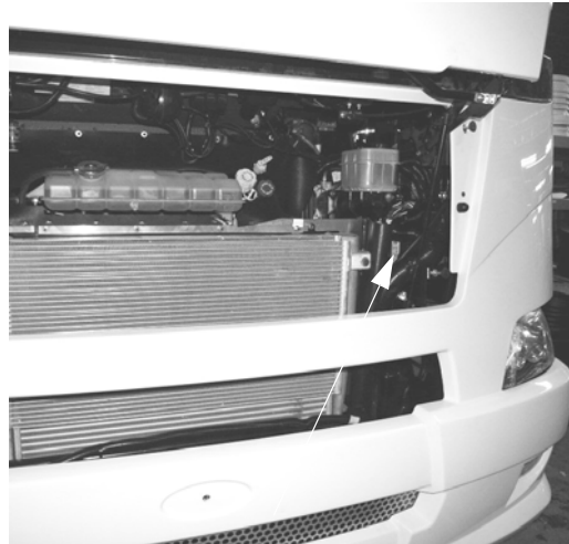
Automotive Fuses (Located behind driver side front hood panel) -Typical View
