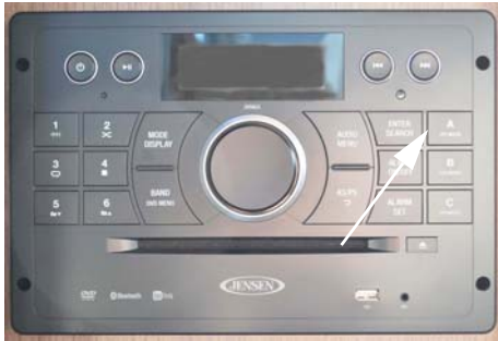
Interior Speaker Switch “SPEAKER A”
