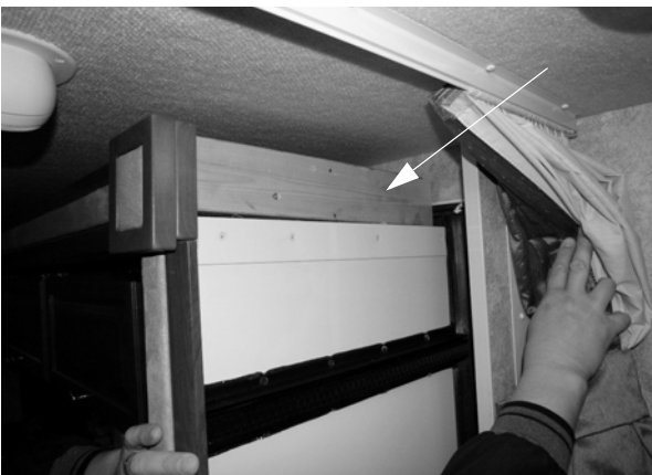
Slideout Travel Support -Typical installation shown
