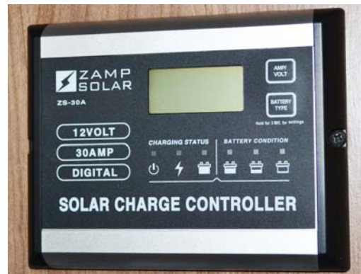
Solar Charge Controller (Located near monitor panel -Typical View
