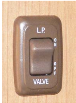
LP Tank Valve Switch
