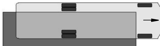
Weighing Right Rear Corner
