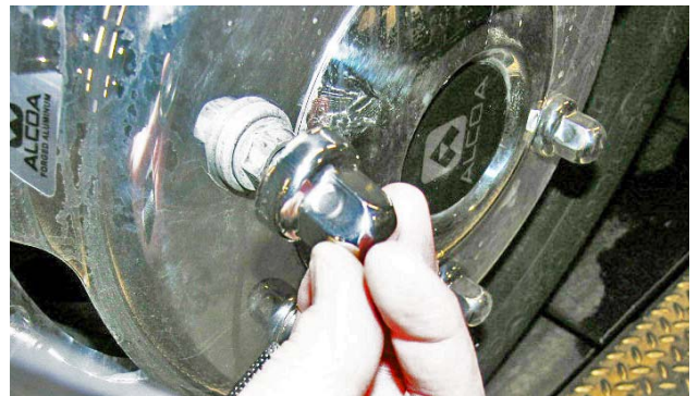
Remove the push on nut covers.
