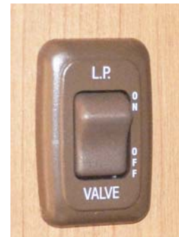
LP Tank Valve Switch
