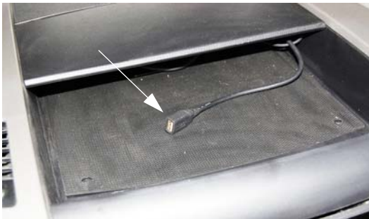
USB Cable (Located in compartment above dash radio) -Typical Installation
