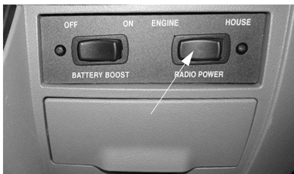
Radio Power Switch (Located on dash)
