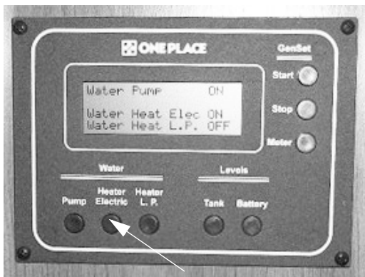
Electric Water Heater Switch (Located on OnePlace® monitor panel)
