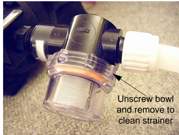
Water Pump Strainer -Typical View
