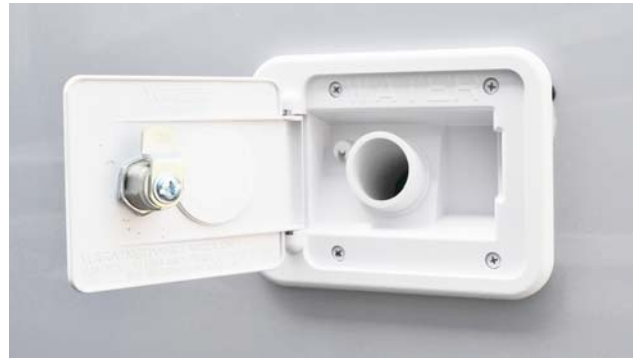
Water Tank Gravity Fill -Typical View
