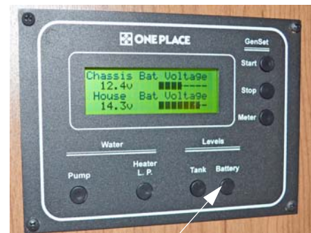
Battery Levels Switch
