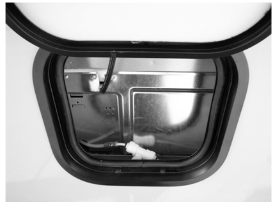
Residential Refrigerator Service Compartment (Located along driver or passenger sidewall, depending on model) -Typical View
