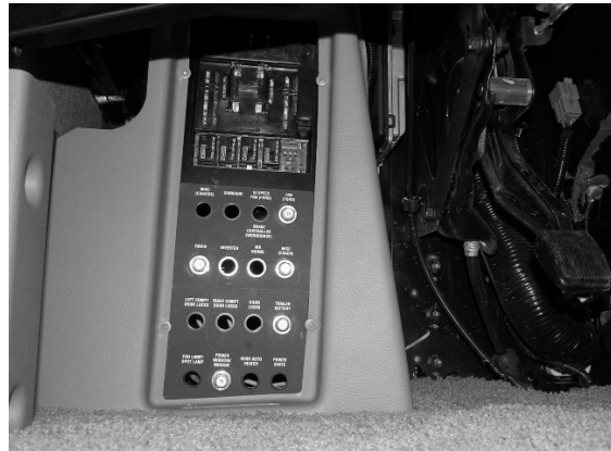
Automotive 12-Volt Circuit Breakers and Fuses (Located beneath left end of dash) -Typical View
