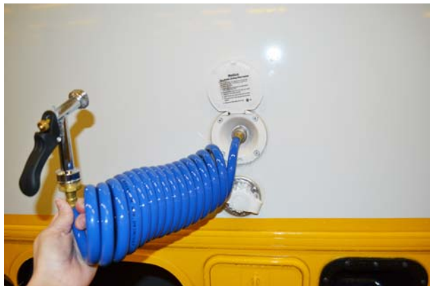
Exterior Shower/Wash Station -Typical View
