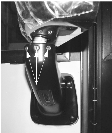
Mirror Head Pivot Lock • Loosen Allen head set screws to pivot mirror head. • Torque 75-100 in./lbs.
