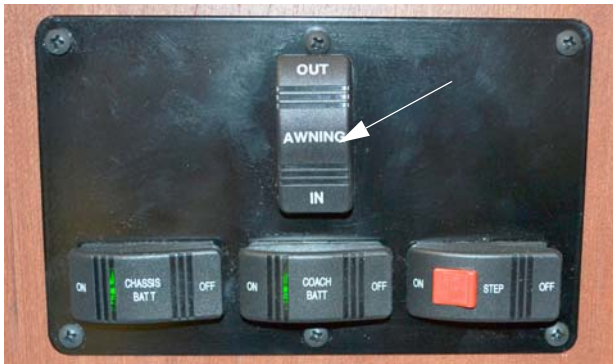
Power Awning Switch (Located near entrance door) -Typical View
