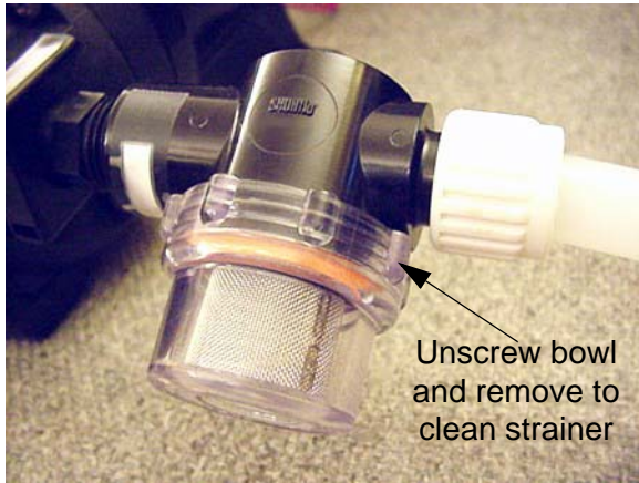
Water Pump Strainer -Typical View
