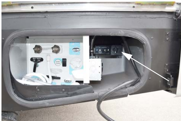
Single Solar Port (Located inside rear driver side exterior compartment) *Models 24G, 24J, and 24V
