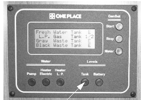
Tank Levels Switch
