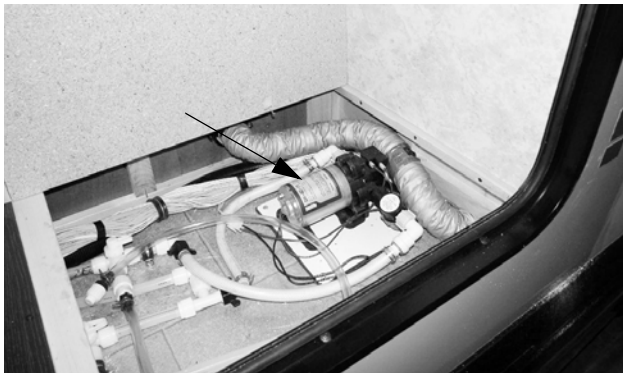
Water Pump (Located beneath removable access panel in passenger rear compartment) -Model 24M shown
