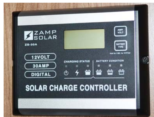
Solar Charge Controller (Located near monitor panel -Typical View
