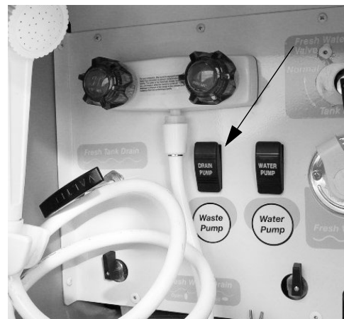
Waste Pump Switch (Located in water service center) -Typical View
