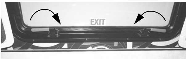
Escape Window (Lift both red safety latch handles UP and push window OUT) -Typical View
