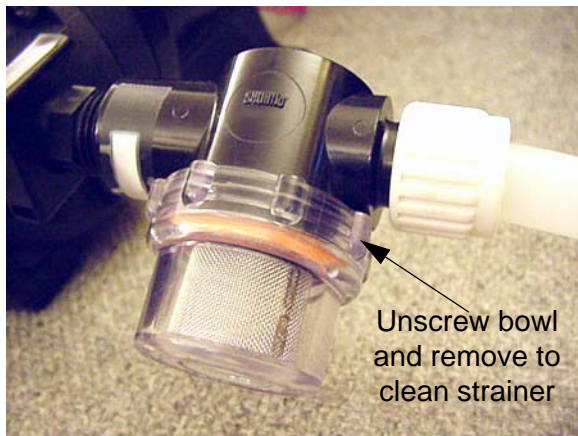
Water Pump Strainer -Typical View
