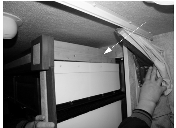
Slideout Travel Support -Typical installation shown • Place support item (e.g. 2x4 wood board) above interior slideout room as shown.
