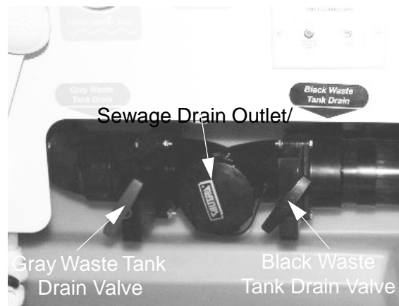
Holding Tank Drain Valves (Located in water service center) -Typical View
