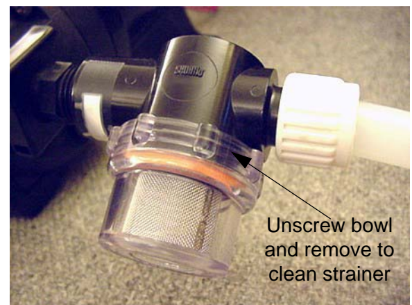
Water Pump Strainer -Typical View
