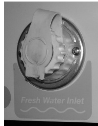
Fresh (City) Water Connection “Fresh Water Inlet” (Located in the water service center)
