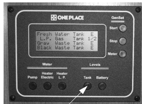
Tank Levels Switch
