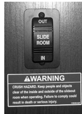
Slideout Switch -Typical View
