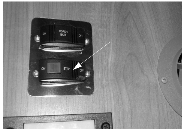
Entry Step Switch (Located near entrance door) -Typical View
