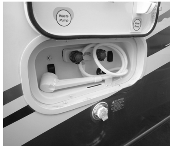
Exterior Shower/Wash Station -Typical View
