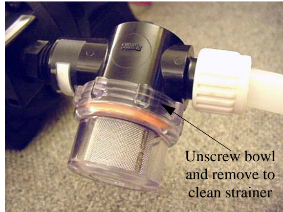
Water Pump Strainer -Typical View
