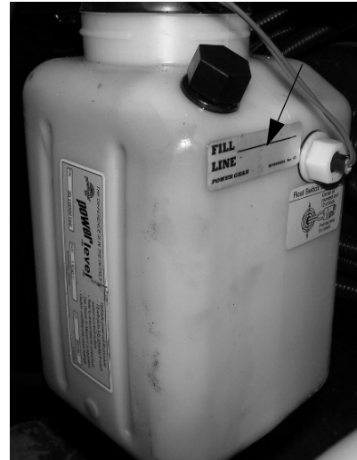
Hydraulic Oil Reservoir -Typical View
