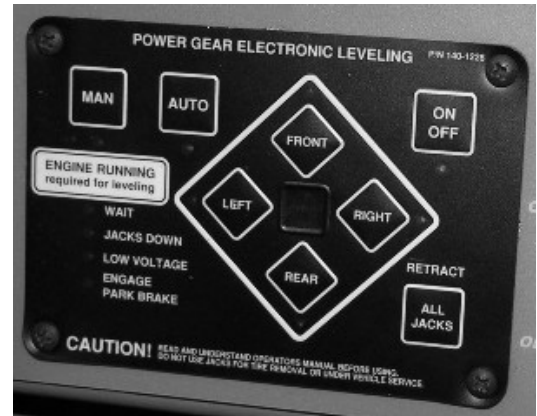
Leveling System Control Panel
