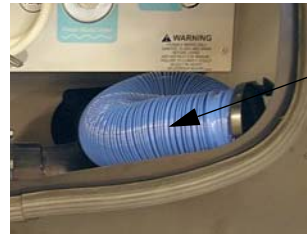
Sewage Drain Hose -Typical View
