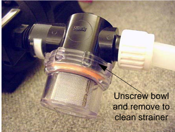
Water Pump Strainer -Typical View
