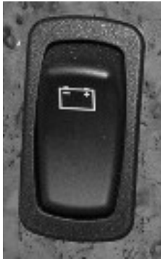
Battery Boost Switch (Located on dash)
