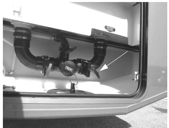
Black Waste Tank Drain Valve (Rear) (Located in water service center) -Typical View
