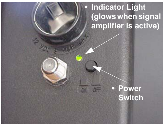
TV Signal Amplifier Power Switch (Located in front overhead cabinet) -Typical View
