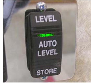
Auto Level Remote Switch (Located inside entrance door) -Typical View
