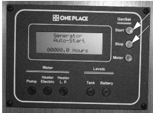
Generator Start/Stop Buttons (Located on monitor panel) -Typical View
