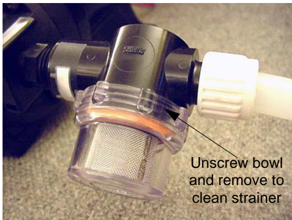
Water Pump Strainer -Typical View
