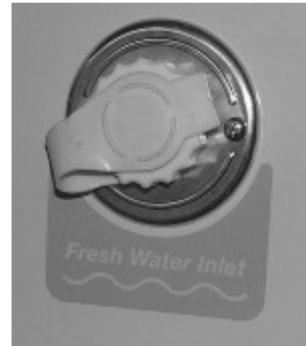
Fresh (City) Water Connection (Fresh Water Inlet)
