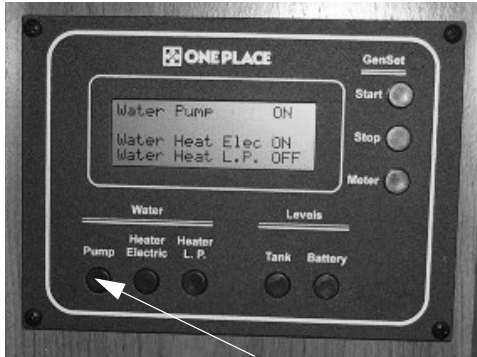
Water Pump Switch
