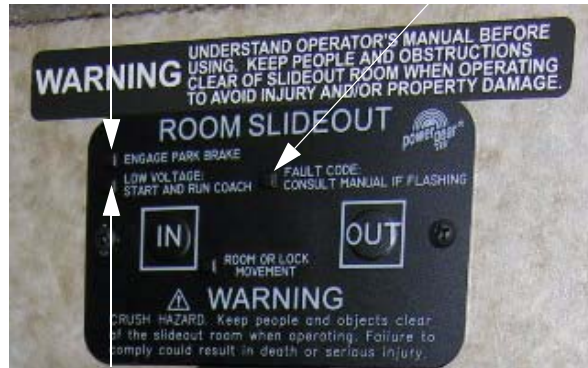
Low Voltage Indicator
