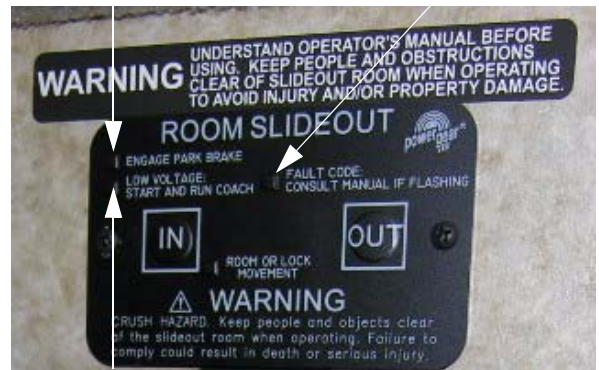
Low Voltage Indicator
