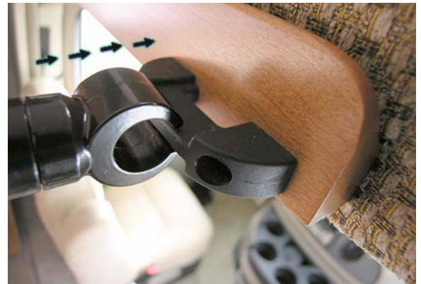
Attaching Bunk Ladder
