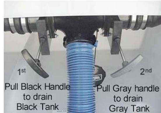
Holding Tank Dump Valves (Typical)
