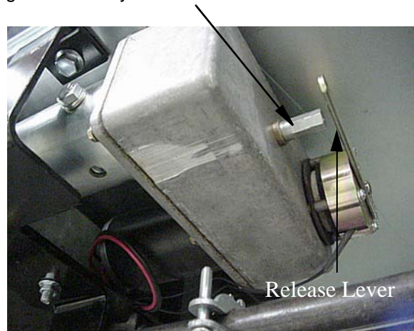
Motor/Gear Assembly (Viewed from the ground)
