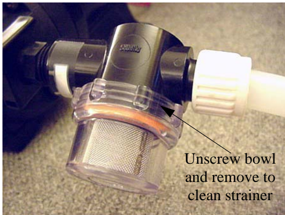
Water Pump Strainer -Typical View
