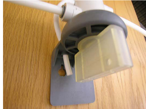
Diverter Plug installed in filter socket. Insert and twist 1/4-turn clockwise, same as filter installation
