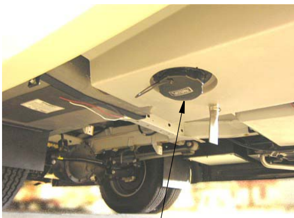
Sewage Drain Outlet (Located on the underside of water service compartment) -Typical View
