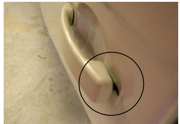
Door Unlatched (note gap)
