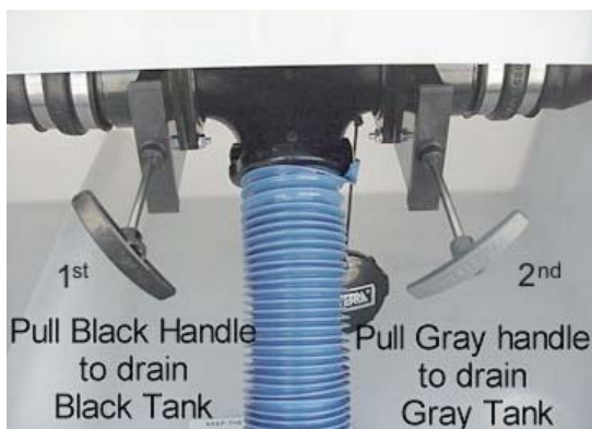
Holding Tank Dump Valves -Typical View
