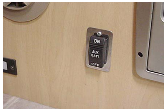
Aux. Batt. Switch - typical (Near entrance door)
