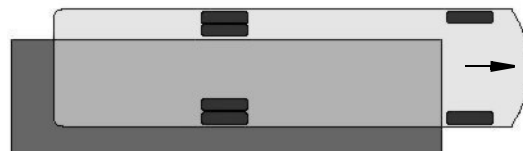
Weighing Right Rear Corner
