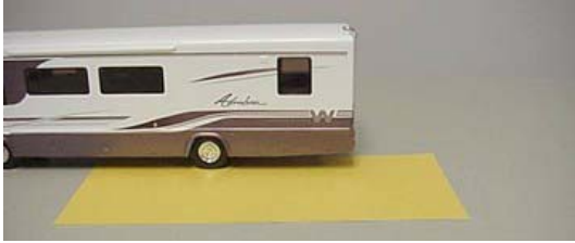
Weighing Left Rear ‘Corner’
