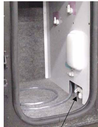
Water Line Drain Valve
