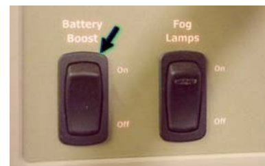
Battery Boost Switch
