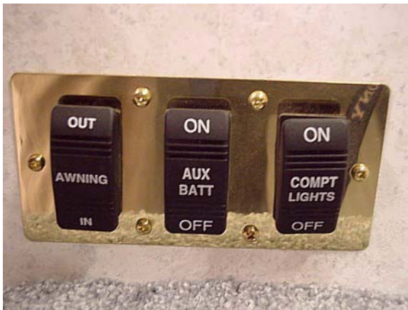
Aux. Batt. Switch (near entrance door)
