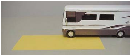
Weighing Left Front 'Corner'
