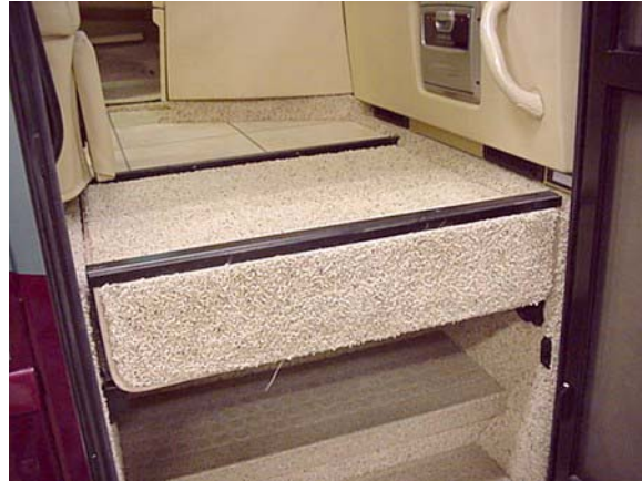
Step Cover shown in extended position
