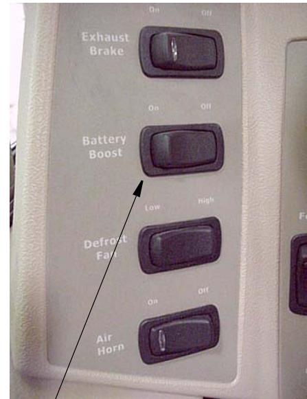
Battery Boost Switch
