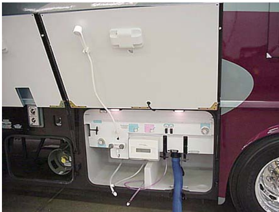
Water Service Center - typical
