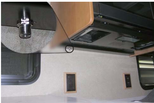
Coaxial connector on underside of range hood on model R36LD with breakfast bar
