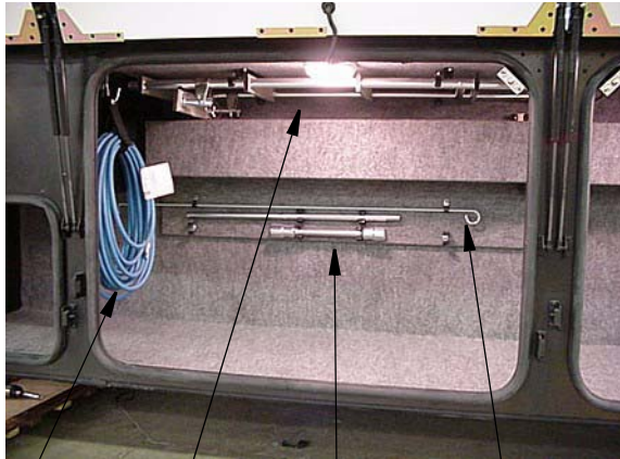
Air Hose Roof Ladder Extension Tire Tools Awning Tool
