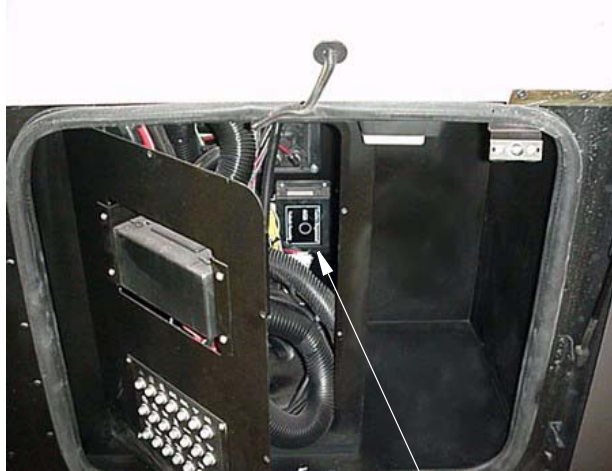
Keyless Entry Control Box in 12-volt electrical compartment.
