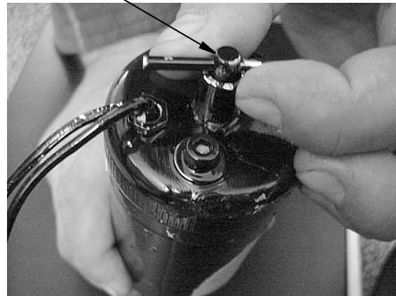
Leveling Jack Solenoid Valve
