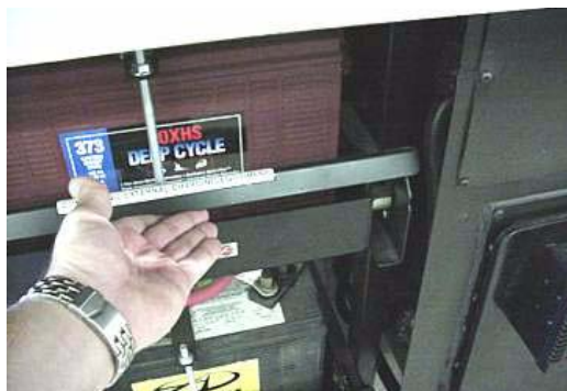
Lift Battery Tray Retainer Latches
