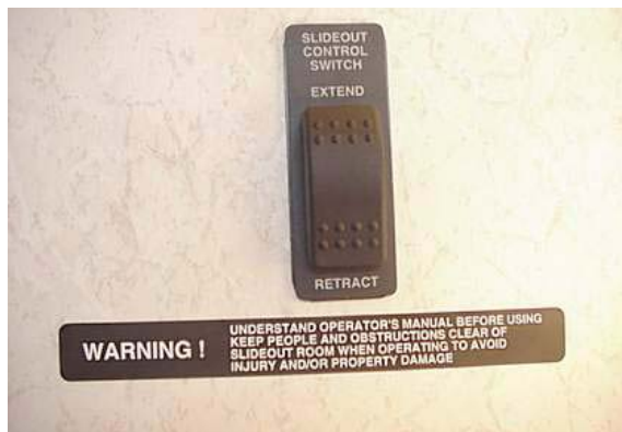
Rear Slideout Switch (on wall in rear of couch - varies by model)
