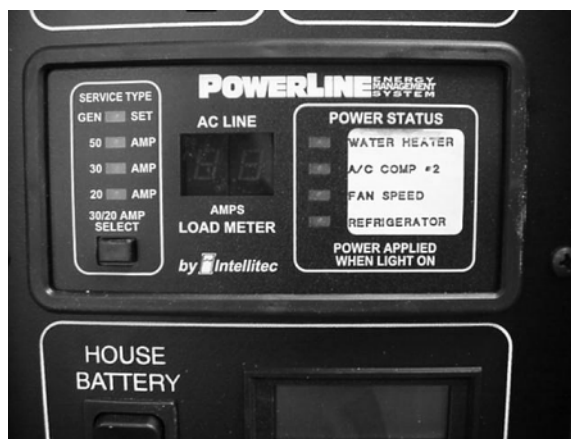
PowerLine EMS Display on OnePlace Monitor Panel
