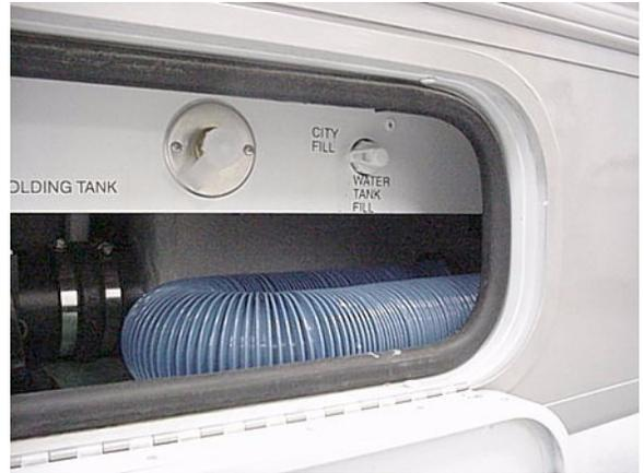
2. Open the Gravity Fill door to provide adequate air venting and avoid pressure buildup.
