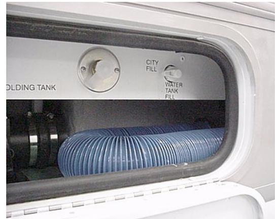
When connected to an outside source of water, the water bypasses the demand pump and storage tank and supplies pressure directly to individual faucets and toilet. A check valve built into the pump prevents water from entering the pump and filling the storage tank.
