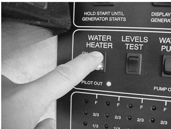
2. If “Pilot Out” light stays on longer than 15 seconds, place switch in “Off” position and wait 5 minutes.
