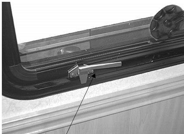
Lift latch handles upward to open.
