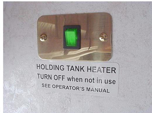
**DO NOT** operate the holding tank heaters unless you are providing a supplemental 12-volt power source to recharge the house batteries. This means either the shoreline cord must be plugged into a 110-volt source, or the auxiliary generator must be operating, or the chassis engine must be running (such as when driving down the road). These three sources can prevent excessive discharge of the house battery.
