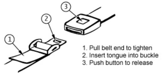
**Adjustment:** To lengthen belt, turn tongue at a right angle to belt and pull to desired length. To shorten, pull loose end of belt.
