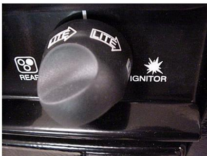
2. While rotating the IGNITOR knob, turn the desired Burner Knob to the LITE position.
