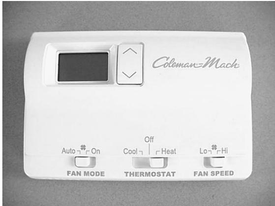
2. Move thermostat switch from OFF to HEAT and press the Temp Selector button (Up/Down arrows) until the desired temperature is shown on the display.
