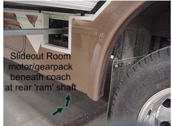
Slideout motor/gear location
