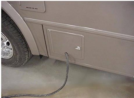
The three-prong power cord is designed to ground the electrical system through the receptacle. It is also designed to carry the amperage output of most campground outlets. If the electrical receptacle to be used is designed to mate with the three prongs on the power cord plug, the electrical connection can be expected to carry rated load. (See approximate power consumption table under generator instructions elsewhere in this section.)
