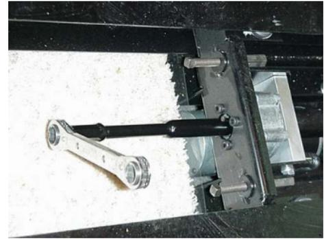
4. The slotted end of the tool must engage with the pin in the endshaft on the slideout gear assembly. See arrow in close-up detail.
