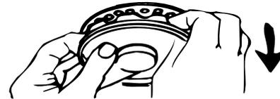
**Lowering Antenna to Travel Position** - Rotate antenna until pointer on rotating knob aligns with pointer on ceiling plate.
