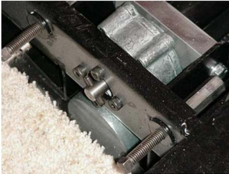
5. Crank the ratched wrench clockwise (to the right) to retract the room. The tool will extend nearly a foot out of the bed base at first, but will be drawn into the bed base as the room is retracted. This is a slow process that will take some time and quite a few turns of the wrench.
